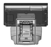
6. Then, slide the cable arrangement cover to remove from the base stand.
