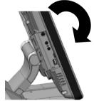
4. With your forefingers, pull by force the locking hook in the direction as indicated by the arrow to remove the neck cover from the base stand.
